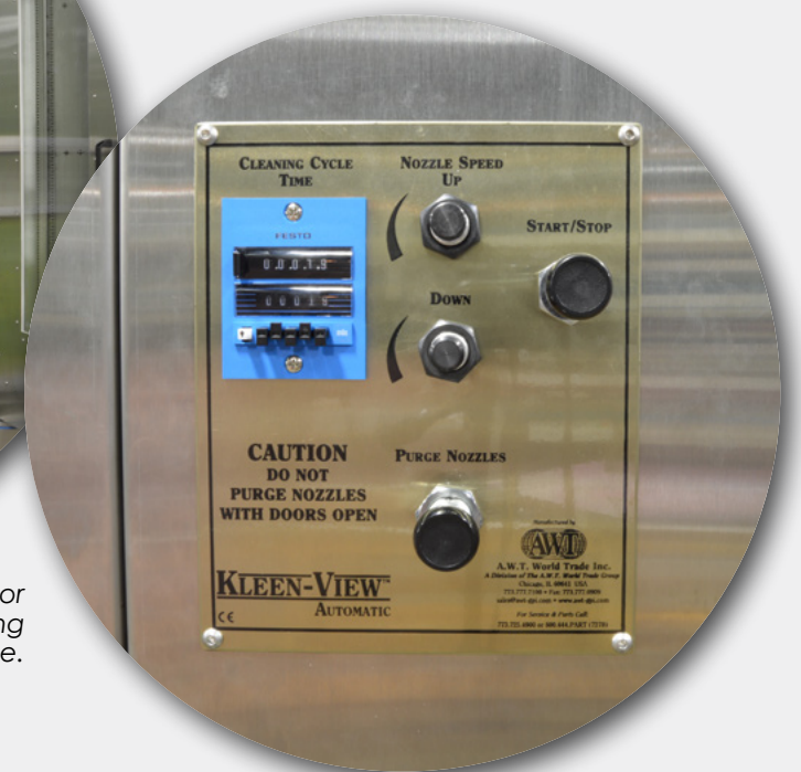
From the convenient control panel, the operator can start/stop cleaning operation, view cleaning time, increase or decrease the nozzle speed and even purge any water remaining in the nozzles.
